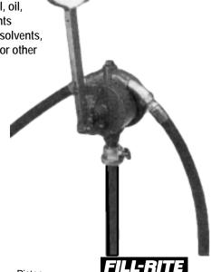
Type Pump: Piston Inlet Size (NPT/in): Outlet Size (NPT/in): 3/4 Delivery Volume (1 gal): 8 strokes Delivery Hose (ID/in): 3/4 Nozzle Type: Straight Inlet Pipe Length (in): 39-1/4 Overall Length (in): 58-1/2
